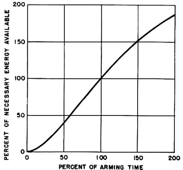
Figure 27. Average arming characteristics of firing condenser.
