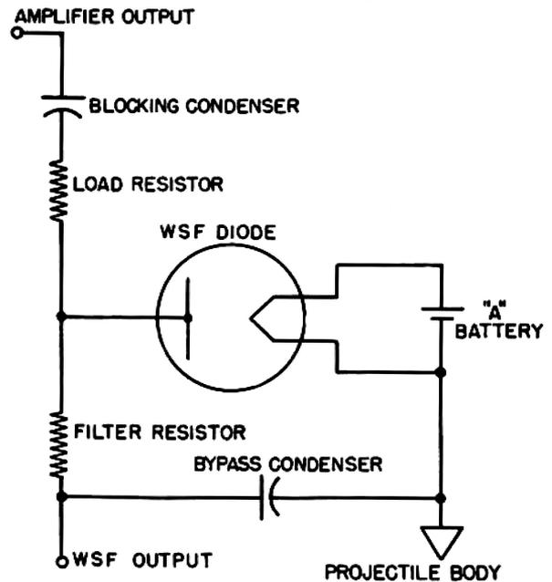
Figure 25. Schematic diagram of wave-suppression-feature (WSF) circuit.
