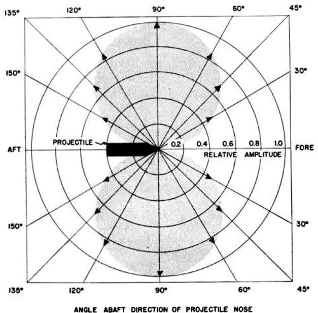
Figure 17. Standard dipole radiation pattern.
