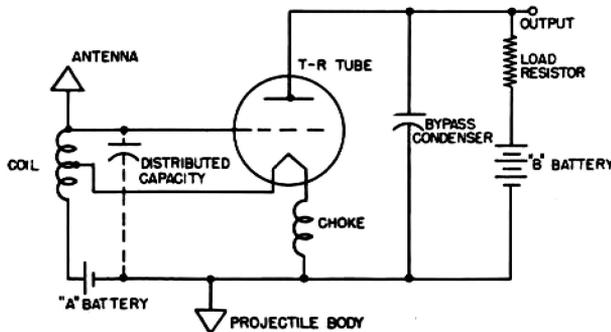
Figure 16. Schematic diagram of transmitter-receiver (T-R) circuit.
