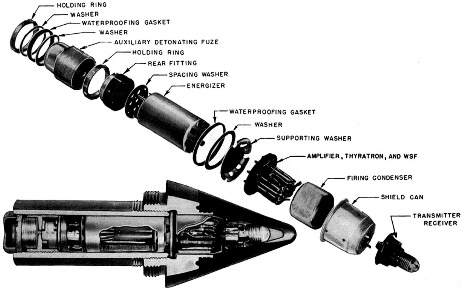
Figure 1. Cutaway and exploded view of a typical VT fuze (VT Fuze Mk 53 Mod 5).
