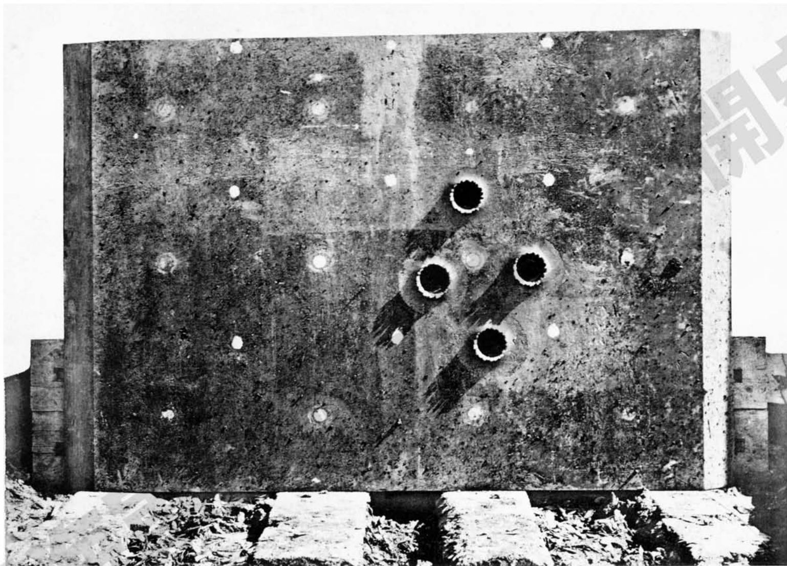
BALLISTIC TEST OF CARNEGIE HOMOGENEOUS NICKEL STEEL ARMOR PLATE, X 20-B. REPRESENTING U. S. ARMORED CRUISER "NEW YORK" 4-INCH SIDE ARMOR. Dimensions 106 x 72 x 4 inches (flat.) Weight 8465 pounds.
